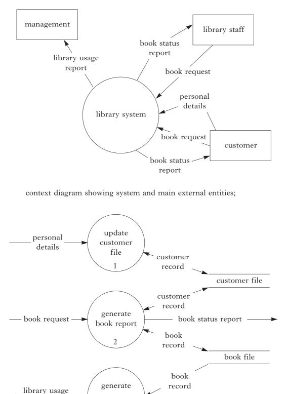
part of data flow diagram showing main processes, files and data flows;
