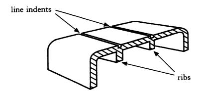
The lid has been produced by injection moulding.
