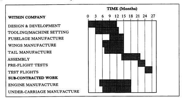
The above project planning chart covers the major stages in the design, manufacture and assembly of a new jet aeroplane.
