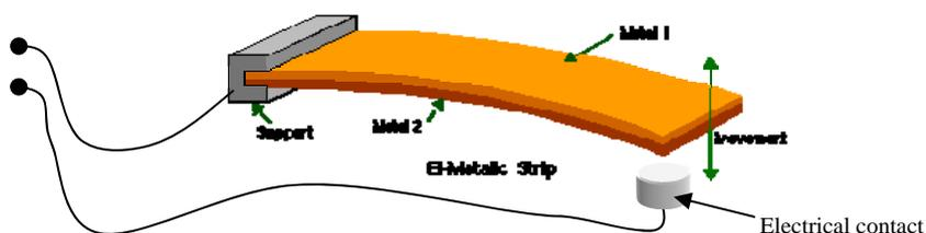
Bi-Metallic Strip – the two metals expand differently for a given temperature rise which results in bending which then operates the electrical contact.
