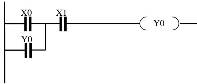
(1 mark for type of contact Y0 and 1 mark for ensuring ONLY the start contact is bridged, not the Paper guard sensor)
