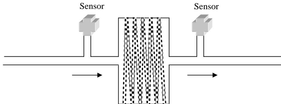
A solution that suggested removing the filter and then making comparative weight or optical density measurements would need to ensure that there are suitable isolation provisions made whilst this is carried out. However any system with a replaceable filter element would need this (or system shut-down) with perhaps hot standby switchover so failure to mention this aspect should not be penalised relative to other factors.
