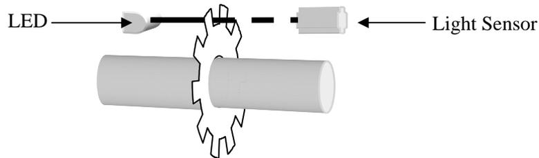
Note: the shredder may rotate in either clockwise or counter-clockwise directions with the additional rotation direction being included to help clear jams. However, it is desirable to detect jams regardless of direction of rotation and hence the simple system suggested.
