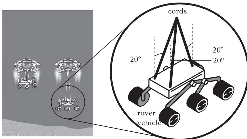
The rover vehicle has a weight of  $1380 \text{ N}$ .
