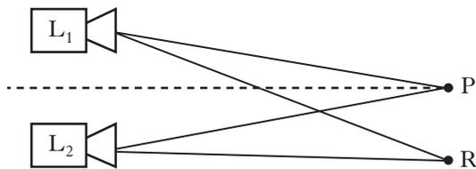
At position P, which is the same distance from both loudspeakers, there is a maximum.
