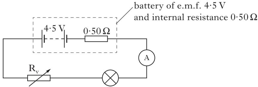
(a) The resistance of variable resistor  $R_v$  is set to  $2.5 \Omega$ . The reading on the ammeter is  $0.30 \text{ A}$ .
