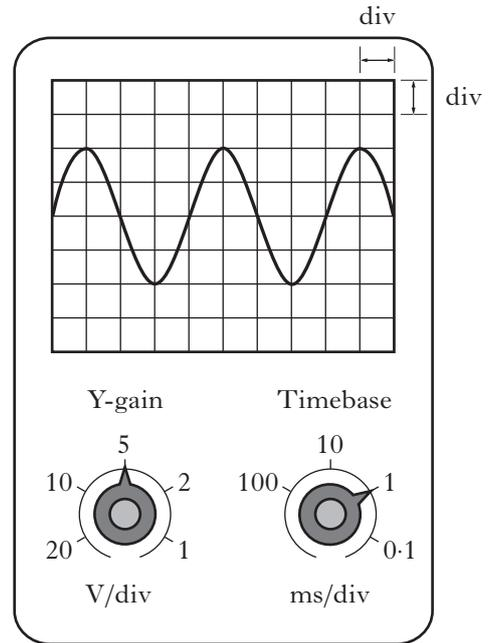
The frequency of the signal shown is calculated using the
