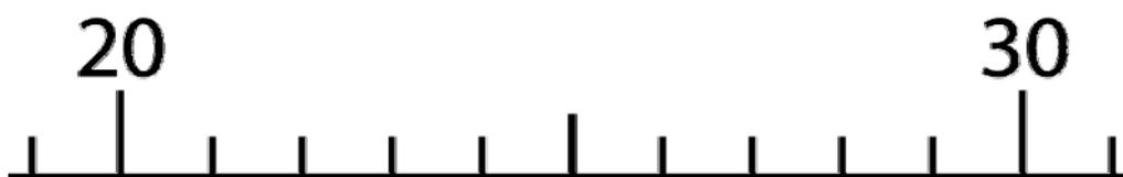
You will need to show the learners how to measure to the nearest division using the convention that if the reading appears exactly half-way between two divisions, the higher value is used.
