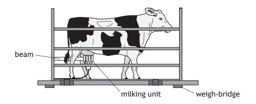
The structural support for the milking unit is considered to be a cantilever beam of length 1.00 m. The milking unit weighs 10 kg and is attached to the free end of the cantilever beam. The beam is made from aluminium alloy and has a hollow rectangular cross-section with external dimensions of width 30 mm and height 70 mm, and a wall thickness of 3.5 mm.
