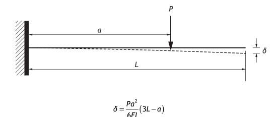
(b) Calculate the vertical deflection of the free end of the cantilever beam that the weight of the cow would produce.
