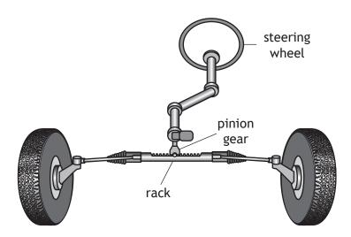
The steering mechanism for an electric car, shown above, comprises a steering wheel connected to a toothed bar, called a rack, via a pinion gear. The pinion gear is fixed in location and is free to rotate. The pinion gear and rack are shown below.
