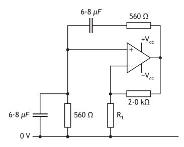
The tolerance of the components used in the circuit is 5%.
