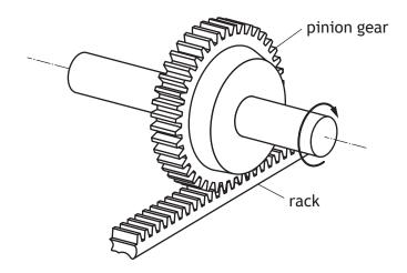
The pinion has a pitch circle diameter of 45 mm and a pressure angle of 25°. A torque of 10 Nm is required at the pinion for the car to turn a corner at a constant speed.
