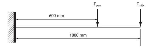
(a) Calculate the maximum stress in the beam at its support and determine if the beam would be permanently deformed if the cow sat down.
