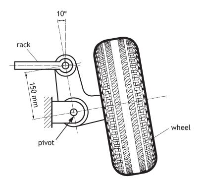
(b) Calculate the required force in the rack to turn the wheels and hence the additional force supplied to the rack by the power steering system.
