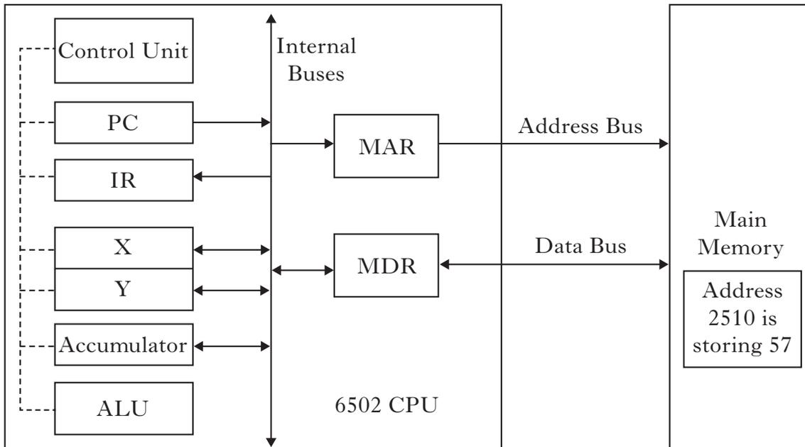
The accumulator, X and Y registers are *general purpose registers*.
