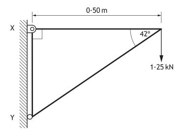
Calculate the magnitude and direction of the reaction at Y.
