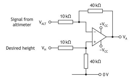
During testing  $\rm V_H$  was changed to  $3\cdot 0\, V$  and  $\rm V_A$  was found to be  $1\cdot 6\, V.$  Calculate the value of  $\rm V_{ALT}$  for this condition.
