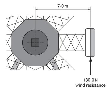
(i) Calculate the torque produced by the drive shaft to overcome the total wind resistance.
