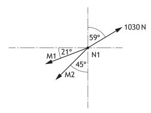
Calculate, using simultaneous equations, the magnitude of the forces in members M1 and M2.
