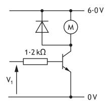
During testing it was found that the motor requires a current of  $97\,\text{mA}$  for the drone to hover. The transistor has a current gain of 210.
