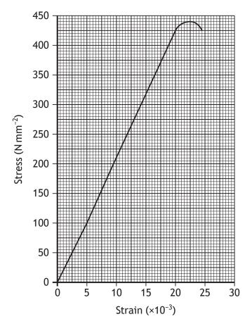
(a) Describe the effect on the specimen of applying and then removing a stress of  $125\,\mathrm{N}\,\mathrm{mm}^{-2}$ .
