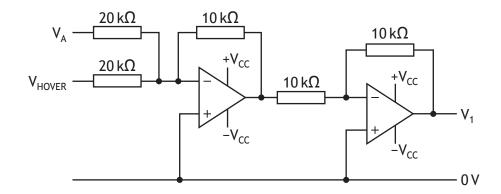
Calculate, using your answer for  $V_1$  the value of  $V_{HOVER}$ . (Assume that  $V_A$  is 0 V at this point).
