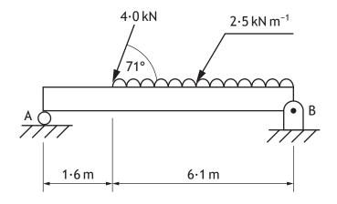
Calculate the magnitude of the reaction at B.
