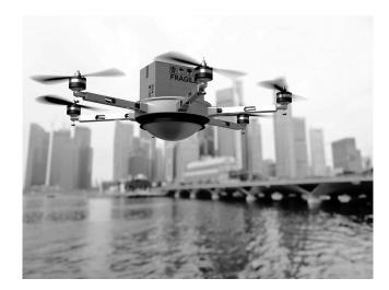
A proportional control system changes the speed of the rotor blades to reach the user's desired height for the drone. An altimeter is used to monitor the current height of the drone.
