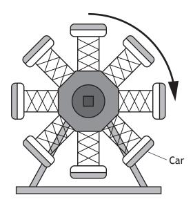
(a) Each of the ride cars is supported by mild steel beams as shown. When the ride is operating the force on a beam was found to be 900.0 N.
