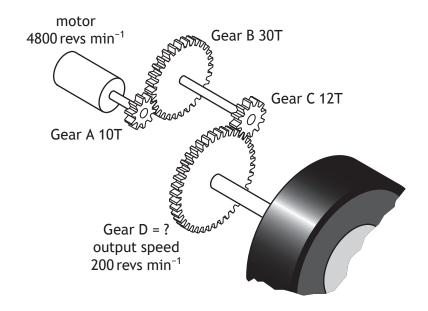
Calculate the number of teeth on gear D.
