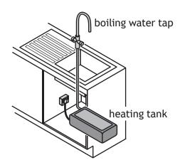
Water is boiled in the heating tank and then stored until it is ready to be used. 1.4 MJ of electrical energy is used when heating a full tank of water for the first time.
