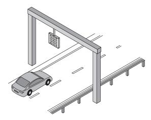
The sign produces a downward force of  $5 \cdot 2 \, kN$  and the weight of the gantry itself is  $22 \, kN$ .
