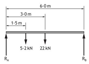
(a) Calculate the reaction force  $R_B$  by taking moments about  $R_A$ .
