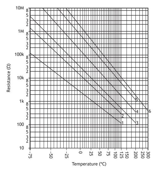
Determine, with reference to this graph, the resistance of the type 1 thermistor at  $40\,^{\circ}\text{C}$ .
