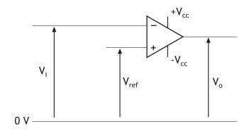
If  $V_i < V_{ref}$ , then  $V_o$  saturates positively (85% of + $V_{cc}$ ) If  $V_i > V_{ref}$ , then  $V_o$  saturates negatively (85% of - $V_{cc}$ )
