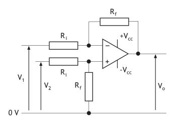
$$A_v = \frac{V_o}{(V_2 - V_1)}$$
