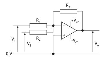
$$A_{v1} = -\frac{R_f}{R_1} \qquad A_{v2} = -\frac{R_f}{R_2} \qquad A_{vn} = -\frac{R_f}{R_n}$$
