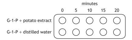
At 5-minute intervals the content of the dimples in each column was tested for the presence of starch.
