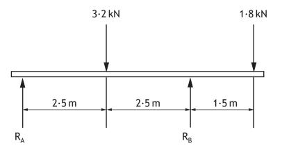
(a) (i) Calculate the size of reaction force  $R_A$ , by taking moments about  $R_B$ . 3
