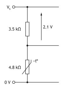
(c) Calculate the supply voltage  $\boldsymbol{V_{s}}$  in the circuit shown above. 4
