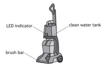
The carpet cleaner uses a heater to maintain the temperature of the water in a clean water tank.
