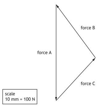
(d) Determine, with reference to the scale drawing shown above, the size of force A.
