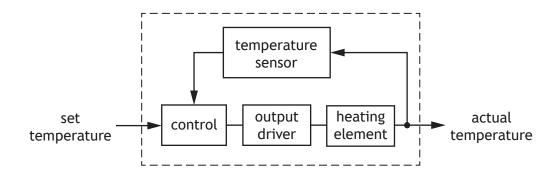
(c) Describe, with reference to the sub-system diagram above, the operation of the system.
