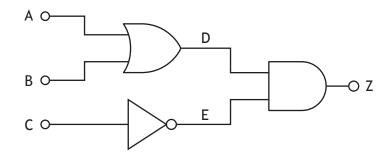
(c) Complete the truth table for the logic diagram shown above.
