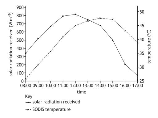
SODIS is most effective when the solar radiation received is above 500 W m<sup>-2</sup> and the temperature is above 45 °C.
