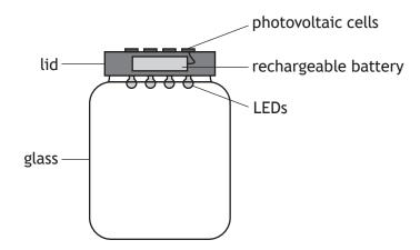
At night, the rechargeable battery is used to power four identical LEDs.
