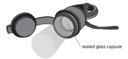
Beta particles emitted by the tritium gas are absorbed by a coating on the inside of the glass capsule.
