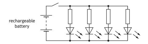
The switch is now closed and the LEDs light.
