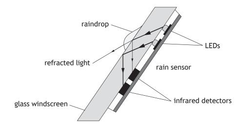
Infrared light is emitted from LEDs and is received by infrared detectors.
