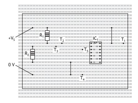
Test points  $T_1$  to  $T_5$  are marked on the stripboard.
