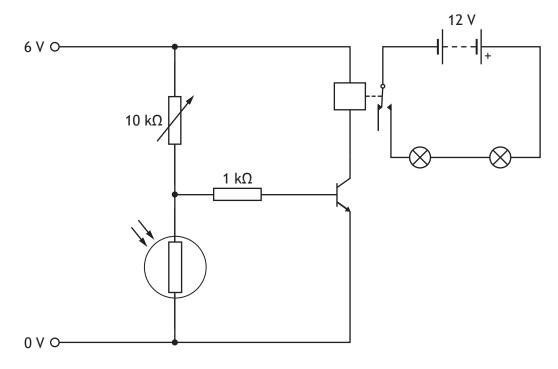
(i) Explain how the circuit operates in order to switch on the car lights when the light intensity falls below a certain value.
