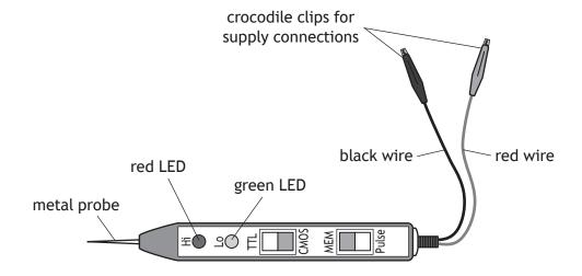
(i) State where the red and black wires should be connected. (a)
