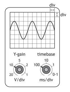
(a) Determine the peak voltage of this signal.
