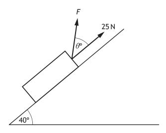
The normal reaction force between the box and the slope is of magnitude 30 newtons. Calculate the angle  $\theta$ °, and the magnitude of the force F.
