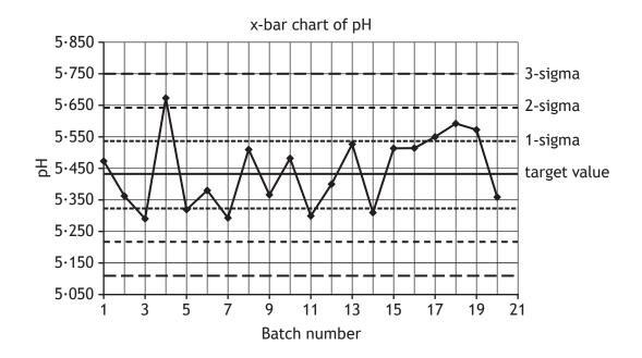
As this is the first time this particular process has been monitored, the first 10 batch means were used to calculate the target pH value and these are listed below.
