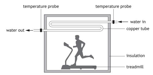
An individual walked on a treadmill in the calorimeter for 30 minutes and the temperature increase of the water was calculated every 5 minutes.
