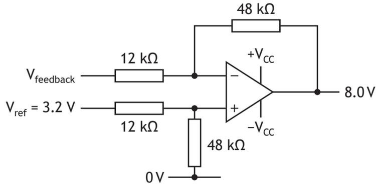
(c) Calculate the voltage from the feedback sensor.
