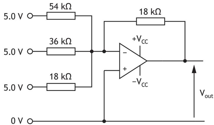
Calculate the output voltage ( $V_{out}$ ) from the operational amplifier (op-amp) shown above.
