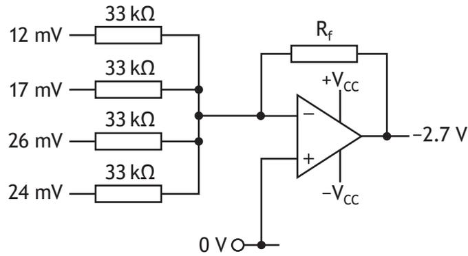
The test circuit above combines the outputs of the four sensors into one signal.
