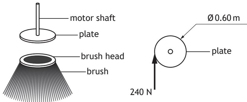
The diameter of the plate is 0.60 m and the force exerted onto the plate when the brush is in motion is 240 N. The motor is rated at 220 V, 6.6 A. Assume the system is 100% efficient.
