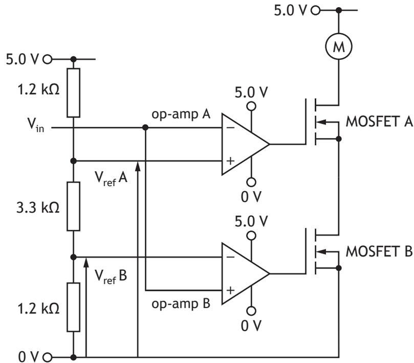
(d) Determine the range of values of  $V_{in}$  that will cause the motor to turn.
