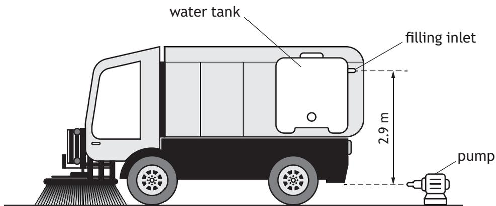
The water tank is filled using an electrical pump, rated at 230 V and 5.0 A. The pump is 87% efficient and the filling inlet is located 2.9 m above the pump.
