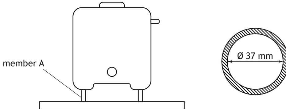
Member A is a tube with an inner diameter of 37 mm. The force from the empty water tank acting vertically on the member is 625 N and the stress present is  $3.4 \text{ Nmm}^{-2}$ .
