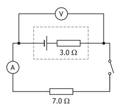
The internal resistance of the cell is 3.0  $\Omega$ .
