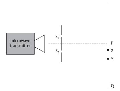
A radiation detector is moved along the line from P to Q.
