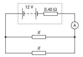
The reading on the ammeter is 4.0 A.
