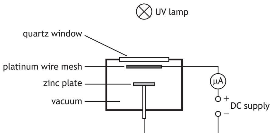
When the lamp is switched on, ultraviolet (UV) radiation passes through the quartz window and wire mesh, and is incident on the zinc plate.
