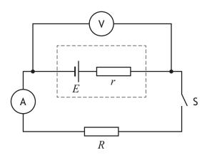
When switch S is open the reading on the voltmeter is  $1.5 \,\mathrm{V}$ .
