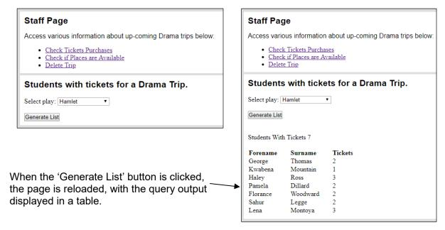
The results of an SQL SELECT statement returns output in the form of an array. The following code was used to display the returned data.
