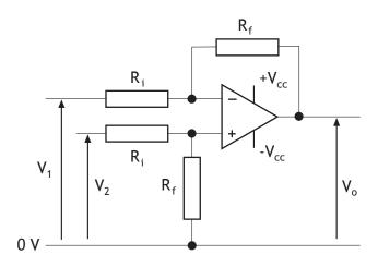
$$A_v = \frac{V_o}{(V_2 - V_1)}$$
