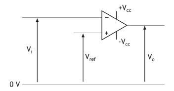
If  $V_i < V_{ref}$ , then  $V_o$  saturates positively If  $V_i > V_{ref}$ , then  $V_o$  saturates negatively
